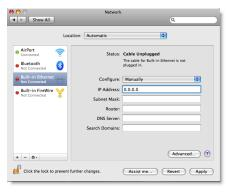
b Enter the IP address details, including the LAN's primary DNS server on the first line in the **DNS Servers** text box.
