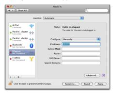
b Enter the IP address details, including the LAN's primary DNS server on the first line in the DNS Servers text box.
