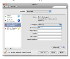
b Enter the IP address details, including the LAN's primary DNS server on the first line in the DNS Servers text box. c If there are any secondary DNS servers, add them on the remaining lines.
